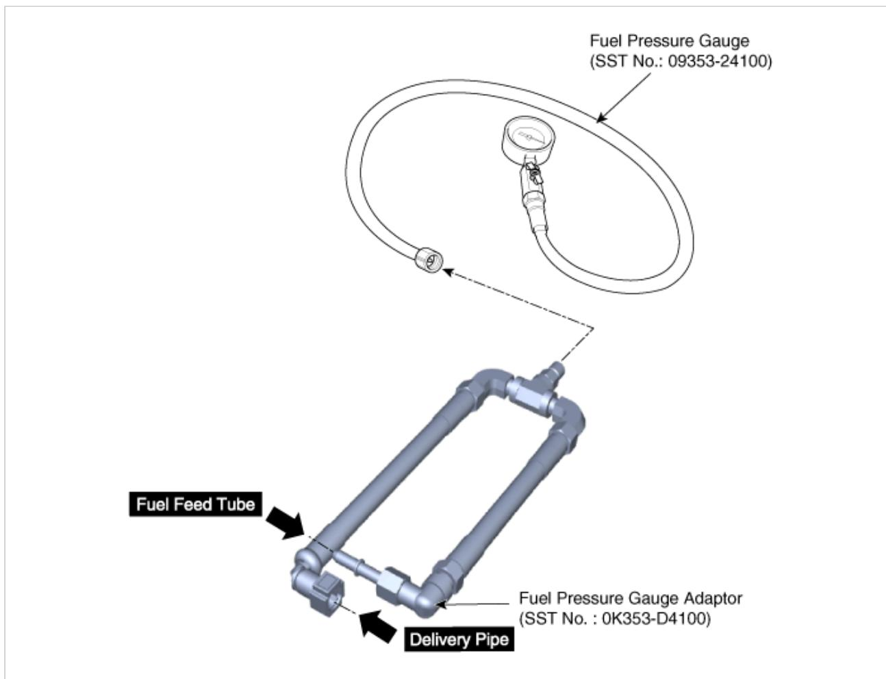
3. Inspect fuel leakage on connections among the fuel feed tube, the delivery pipe, and the SST components with ignition "ON".
